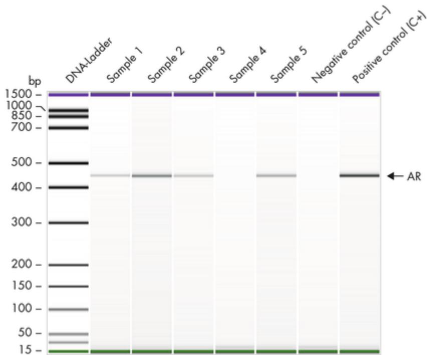
**Figure 4. AdnaTest ProstateCancerDetect results of singleplex PCR samples.** The first lane shows the DNA size standard (DNA-Ladder). Samples 1 to 3 and sample 5 are positive for AR. Sample 4 is negative. The PCR negative (C-) and positive control (C+) are shown in the last two lanes.
