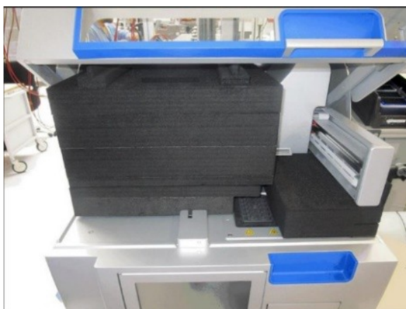
Foam protector above centrifuge.
