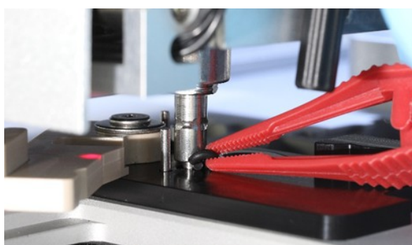
Open the gray lever and remove the O-Ring using the tweezers.
