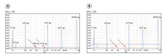
Figure 4. A The threshold is used during peak detection. Signals that exceed the threshold value (dark blue line) are detected as peaks. B If non-relevant peaks are identified, the threshold can be increased (e.g., to 5 %) to exclude the non-relevant or unspecific data from the analysis.
