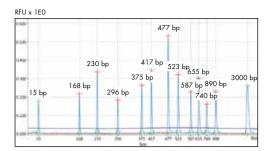
Figure 2. Electropherogram of the control sample from lane 12. All 11 amplicons used for identification are clearly visible and well separated. Peaks at 15 bp and 3000 bp correspond to alignment markers.
