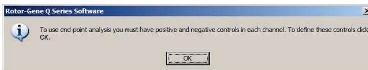
Click **OK**. The **Edit Samples** window appears, allowing positive and negative controls to be defined. To define a sample as a positive or negative control, click on the sample type cell, then select the relevant control type from the drop-down menu.
