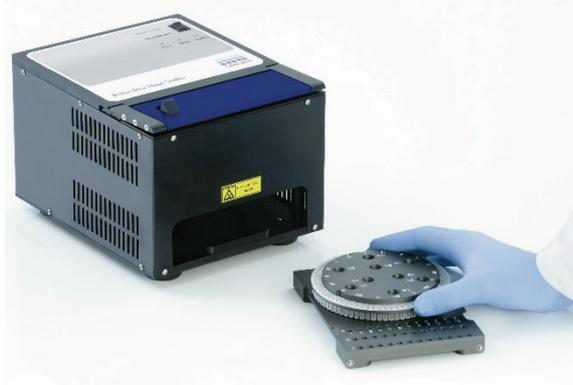
5. Remove the central portion from one sheet of Rotor-Disc Heat Sealing Film by slightly folding the film in half, pinching the center piece, and carefully tearing it out.
