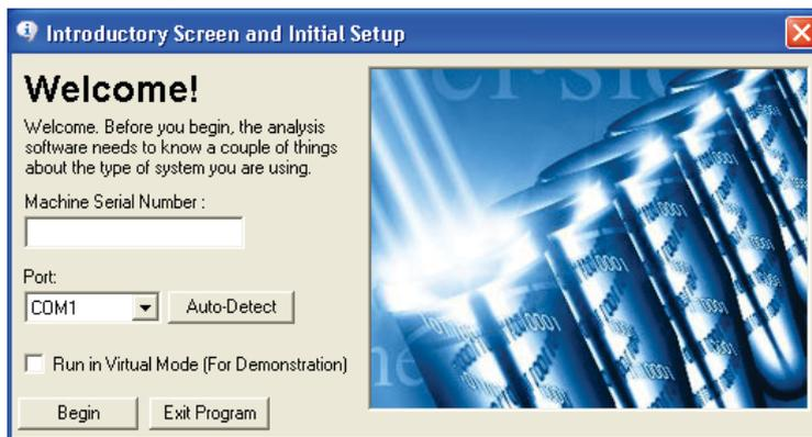
**Machine Serial Number:** Type in the serial number (7 digits), which can be found on the back of the Rotor-Gene Q MDx.
