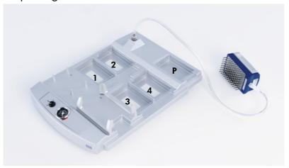
Placement of PCR plate (or strips) and PyroMark Q96 HS Plate (PM Plate) on the PyroMark Q96 Vacuum Workstation. The marked positions contain 70% ethanol (1), PyroMark Denaturation Solution (2), PyroMark Wash Buffer (3), and high-purity water (4 and P).
