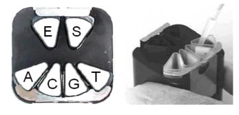
**Arrangement of tips in the PyroMark Q96 Capillary Tip Holder. E**: Enzyme Mixture; **S**: Substrate Mixture; **G**: dGTP; **C**: dCTP; **T**: dTTP; **A**: dATPαS.
