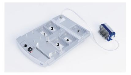
Placement of PCR plate (or strips) and PyroMark Q96 Plate Low (PM Plate) on the PyroMark Q96 Vacuum Workstation. The marked positions contain 70% ethanol (1), PyroMark Denaturation Solution (2), PyroMark Wash Buffer (3), and high-purity water (4 and P).
