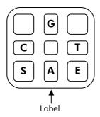
**Schematic diagram of the PyroMark Q96 Cartridge (viewed from above). E**: Enzyme Mixture; **S**: Substrate Mixture; **G**: dGTP; **C**: dCTP; **T**: dTTP; **A**: dATPαS.
