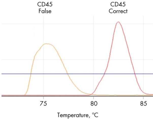
**Figure 4. Example melting curves.** The left curve shows an incorrect melting temperature for the given PrimerMix. Melting curves should be Gaussian-like, with a clear maximum at the melting temperature.
