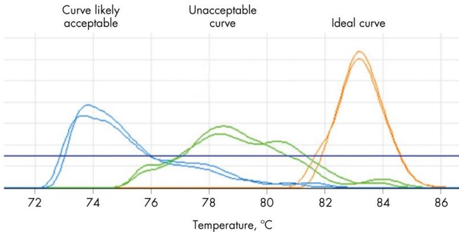
**Figure 5. Example melting curve shapes.** The green curve is unacceptable and results should be excluded. The blue curve shows a suboptimal shape, but if the melting temperature is correct, then results can be accepted. The yellow curve shape is optimal, and results can be accepted if the melting temperature is also correct.
