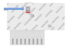
Figure 4. Sample inspection window (blue arrow).
