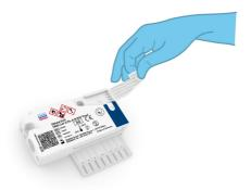
Figure 19. Opening the sample lid of main port.
