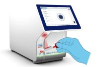
Figure 24. Scanning sample ID bar code.
