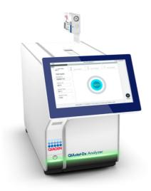
Figure 15. Inserting QIAstat-Dx SARS-CoV-2/Flu A/B/RSV Panel Cartridge into QIAstat-Dx Analyzer 1.0 or the QIAstat-Dx Analyzer 2.0.
