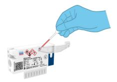
Figure 21. Transferring sample to main port of QIAstat-Dx SARS-CoV-2/Flu A/B/RSV Panel Cartridge.
