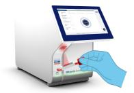
Figure 11. Scanning sample ID bar code.
