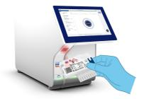
Figure 12. Scanning QIAstat-Dx SARS-CoV-2/Flu A/B/RSV Panel Cartridge bar code.
