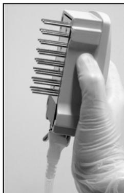
Figure 10. Illustration of the vacuum tool raised to beyond 90° vertical.
