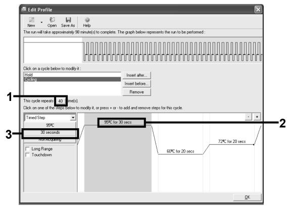
Figure 6. Cycling step at 95°C.
