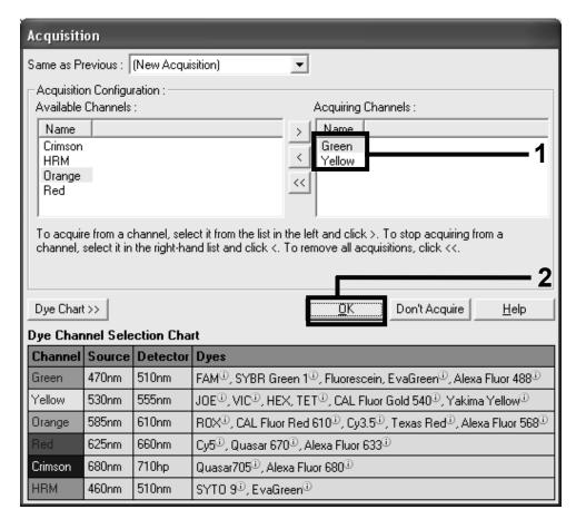
Figure 8. Acquiring at cycling step of 60°C.
