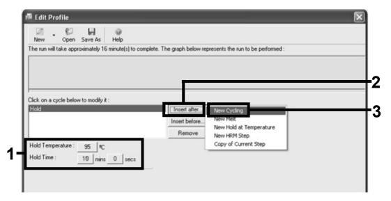
Figure 5. Initial incubation step at 95°C.
