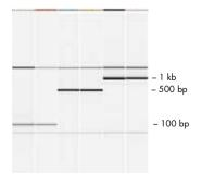
Figure 4. Highly specific amplification using QIAGEN Tag DNA Polymerase and clear separation of fragments using the QIAxcel. PCR was performed to amplify 3 different fragments (corresponding to 100 bp, 500 bp, and 1 kb). Reactions were run in duplicate. The QIAxcel enabled clear separation of the fragments.
