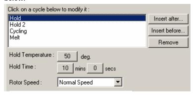
3. Select "Hold2" and set up the parameters for the initial activation step as shown below.
