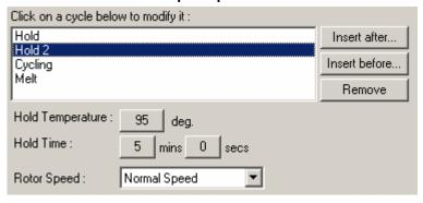
4. Select "Cycling" and set up the parameters for PCR cycling as shown below.
