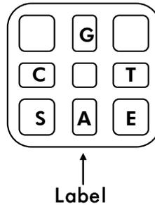
**PyroMark Q96 Cartridge (from above) with indicated compartments for enzymes, substrate, and nucleotides.**
