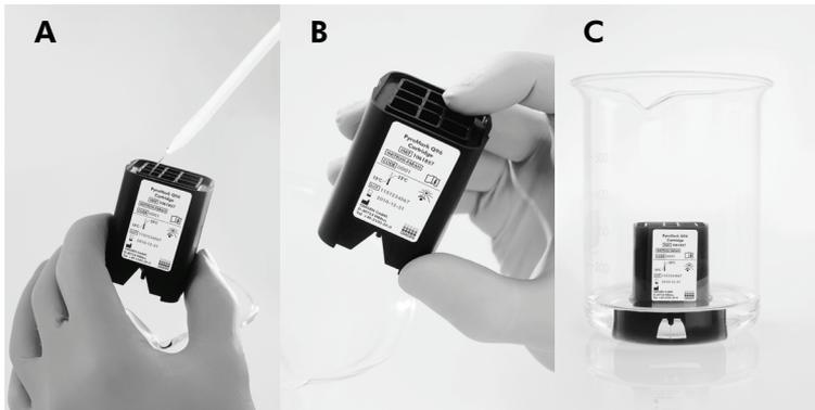
**Cleaning the PyroMark Q96 Cartridge.** **A** Filling the compartments with high-purity water. **B** Placing pressure on compartments. **C** Cartridge immersed in a beaker with high-purity water.
