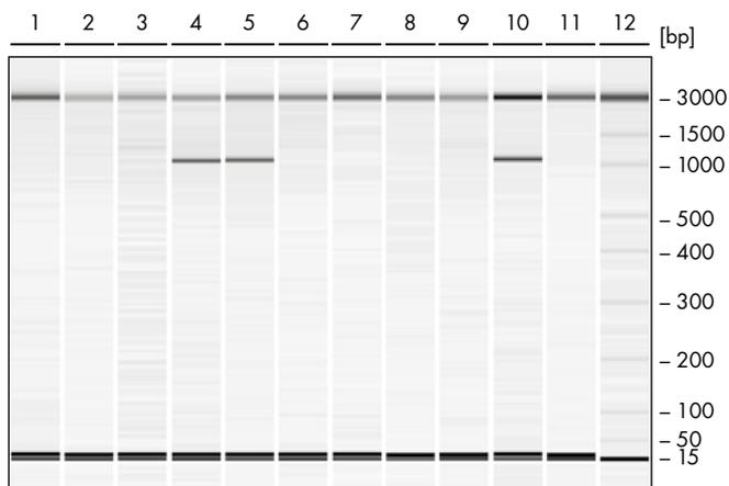
**Figure 3.** PCR product analysis of TEM beta-lactamases in *E. coli* isolates on QIAxcel. Lanes 1–3 and 6–9 contain negative samples, lanes 4 and 5 positive samples, lane 10 a positive control, and lane 11 a negative control. Lane 12 displays the DNA size marker 50 bp–1.5 kb.
