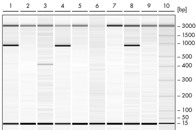
**Figure 4.** PCR product analysis of CTX-M-1 group beta-lactamases in *E. coli* isolates on QIAxcel. Lanes 1 and 4 contain positive samples, lanes 2, 3, 5-7 negative samples, lane 8 a positive control, and lane 9 a negative control. Lane 10 displays the DNA size marker 50 bp–1.5 kb.
