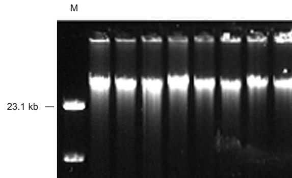
**Figure 2.** Agarose gel analysis of 400 ng DNA (0.5% agarose gel, 1 x TAE buffer, 23 V, 16 h; for optimal separation of high-molecular-weight DNA) purified from blood samples from 8 donors after storage in PAXgene Blood DNA Tubes for 7 days at 30°C. **M:** Marker.
