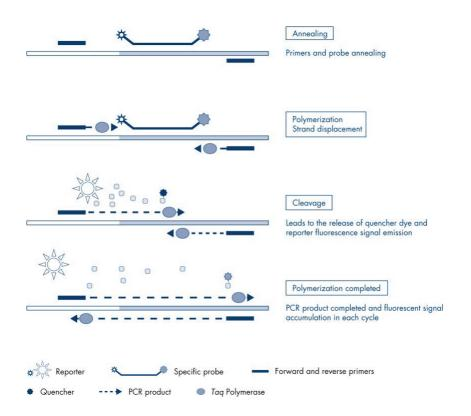
Figure 2. Reaction principle with hydrolysis probes.
