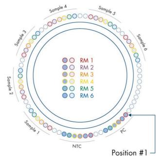
Figure 5. Plate and rotor setup for an experiment with the PIK3CA RGQ PCR Kit. PC: Positive Control. S: DNA sample. NTC: No-template control (water).
