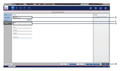
Figure 11. Create work list main window. 1 = "Properties" tab, 2 = Entering worklist name, 3 = Select "is editable" and the "work list is complete", 4 = "Apply".
