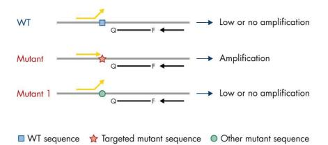
Figure 1. Identification of specific mutation by ARMS PCR. WT: Wild type. Q-F: Double-dye probe.  $\Rightarrow$ : Forward and reverse primers.
