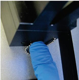
3. Press the sliding security bolt into the side slot opening.
