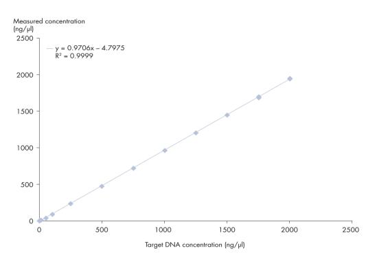
Figure 2. Excellent measurement linearity of QlAxpert. The spectrophotometry data were plotted against the target concentration. The data demonstrate outstanding linearity for samples with concentrations up to 2000 ng/ $\mu$ l or 40 OD ( $A_{260}$ , 10 mm), respectively. The calculated regression coefficient is >0.999.
