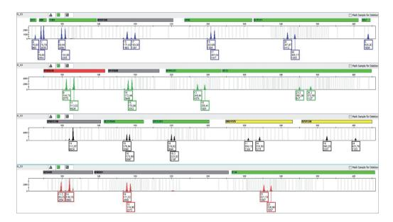
Figure 6. Example electropherogram using the Investigator Casework GO! Kit showing a balanced profile with no signs of inhibition.
