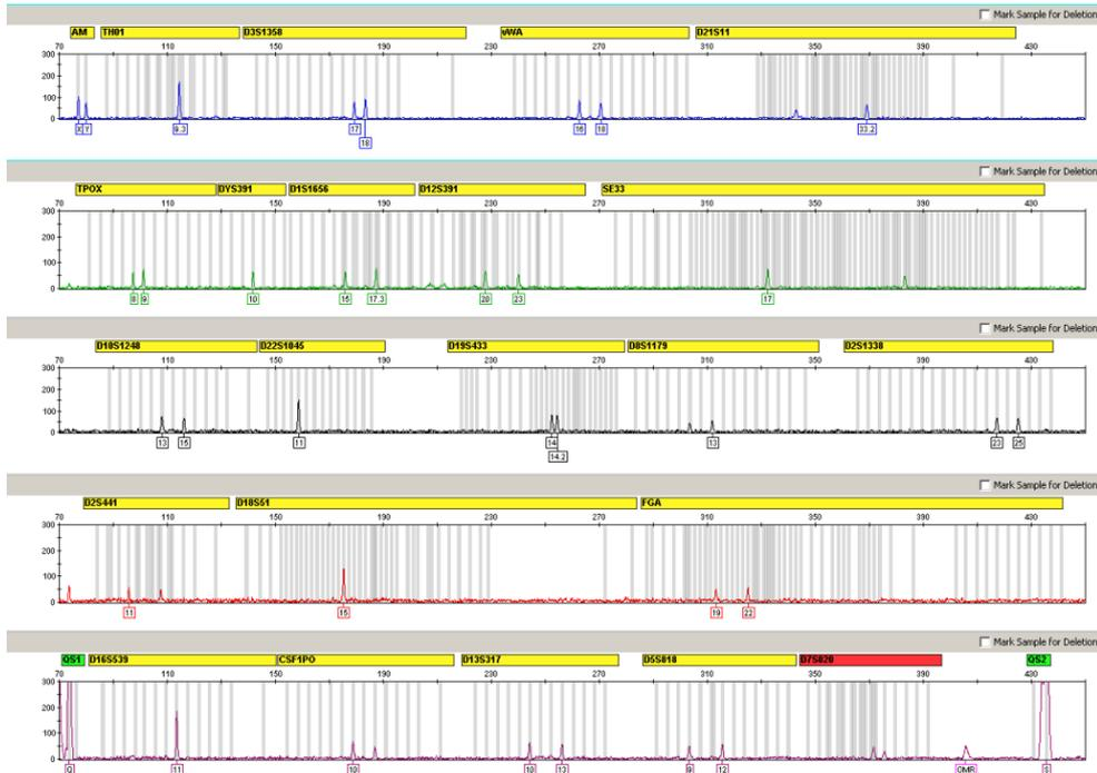
**Figure 9. Sensitivity study.** Example of a blood on FTA sample using blood that has been diluted 1:9-fold prior to spotting. Several alleles dropped below 50 RFU.
