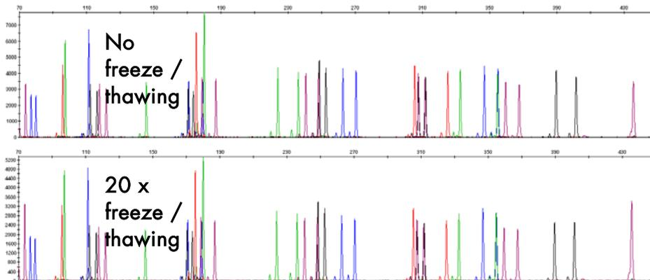
Figure 41. Results of a simulated freeze / thawing stability test of kit components.
