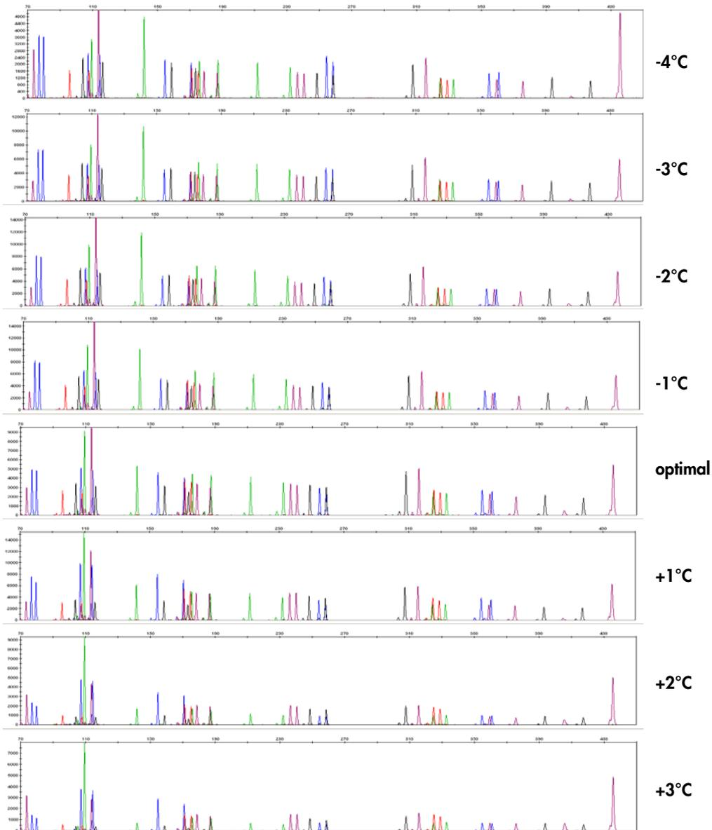
**Figure 4. Variations in the PCR annealing temperature.** Blood on FTA samples were amplified on an Eppendorf Mastercycler ep. Representative electropherograms for reactions using annealing temperatures between -4°C and +3°C are shown. Note that the y-axis was scaled for best fit.
