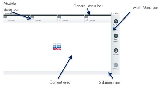
Figure 41. Main screen of the QIAstat-Dx Analyzer 1.0 touchscreen.
