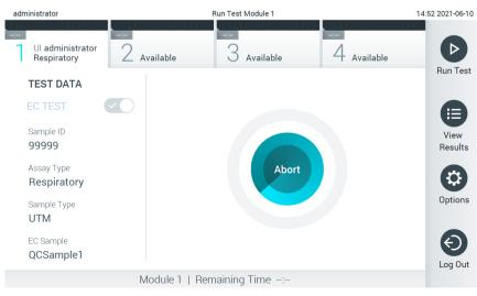
Figure 95. Test execution and remaining run time display.
