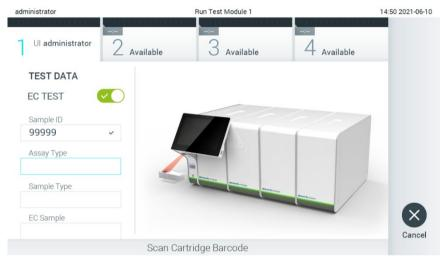
Figure 90. Scanning the QIAstat-Dx assay cartridge bar code.
