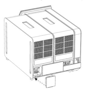
Figure 19. Connecting the Termination Bridge.
