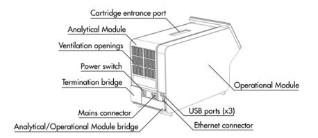
Figure 2. Rear view of the QIAstat-Dx Analyzer 1.0. The Operational Module is on the right and the Analytical Module is on the left.
