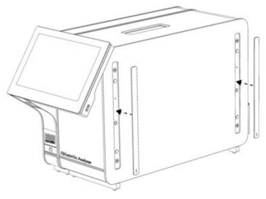
Figure 7. Reattaching the protective covers.
