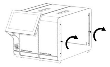
Figure 16. Aligning and attaching the additional Analytical Module.
