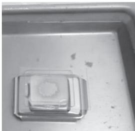
Fill a cryomold with cryo-embedding medium and pre-cool in 2-methylbutane.
