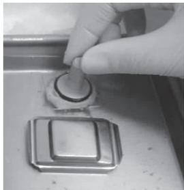
Completely submerge the cryomold with tissue into the 2-methylbutane.
