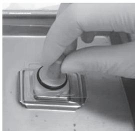
Immediately place a specimen disk on top of the cryo-embedded tissue.
