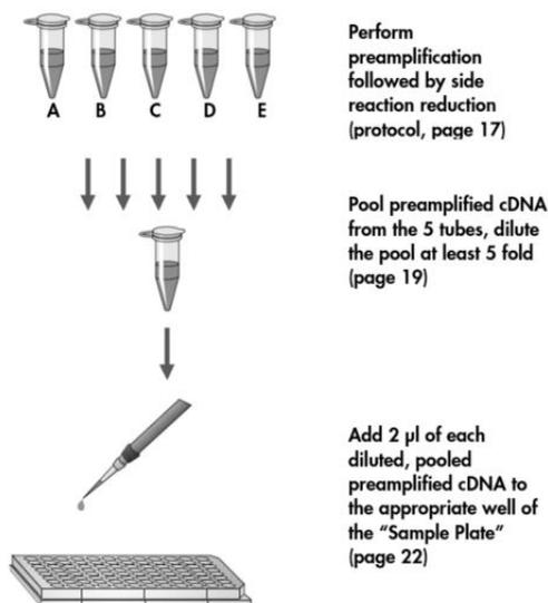
**Figure 2. Preamplification using miScript PreAMP miRNome Primer Mixes in multiple tubes.** Preamplification reactions are set up for each tube of primer mix, and the preamplified cDNA is then pooled and diluted at least 5-fold prior to being aliquoted into the sample plate.
