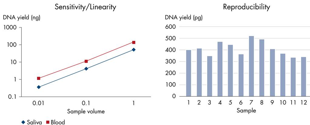
**Figure 2. Sensitivity and reproducibility of the Investigator STAR Lyse&Prep Kit.** Data was generated using the 300 µl protocol on the Hamilton® STAR Instrument.
