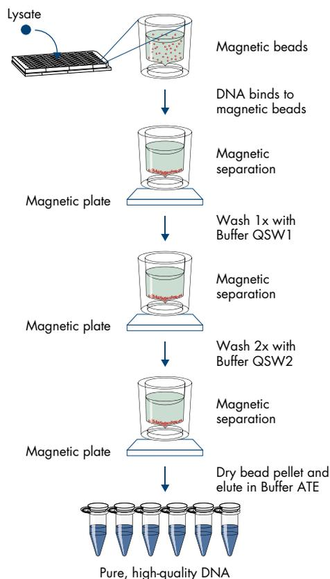
**Figure 1. Schematic procedure of the sample prep workflow using the Investigator Lyse&Prep Kit on an open DNA extraction platform.**
