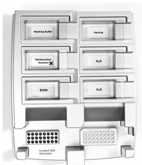
**Figure 2.** Placement of PCR plate and PyroMark Q24 plate on the vacuum workstation.
