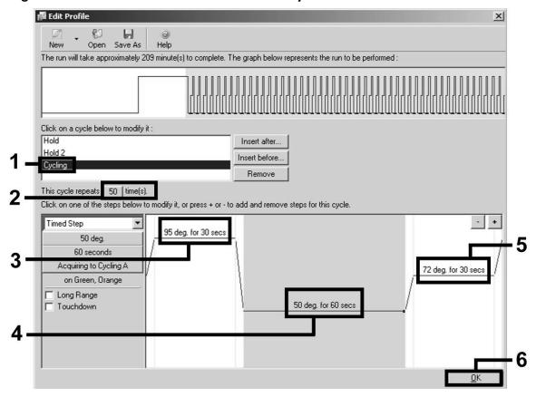
**Figure 9. Amplification of the cDNA.** Note that, on the Rotor-Gene 3000, the software will define the fluorescence dyes as "FAM/Sybr, ROX".
