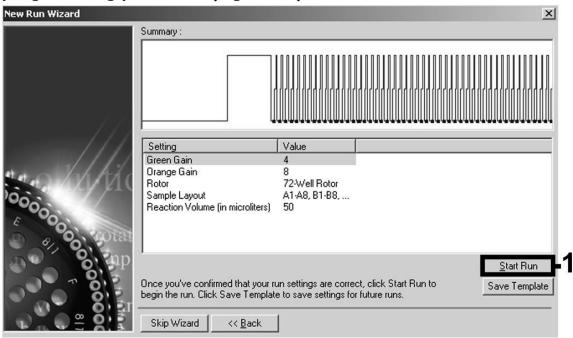
**Figure 11. Starting the run.** Note that, on the Rotor-Gene 3000, the software will define the fluorescence dyes as "FAM/Sybr" and "ROX".
