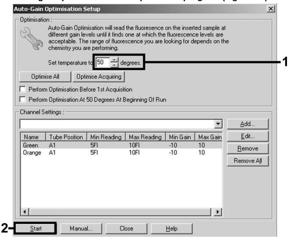
**Figure 10. Adjusting the fluorescence channel sensitivity.** Note that, on the Rotor-Gene 3000, the software will define the fluorescence dyes as "FAM/Sybr" and "ROX".
