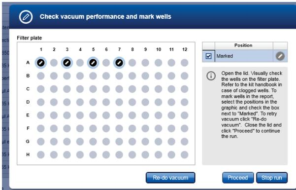
4. If liquid still remains in any well, manually remove the liquid using a pipet.
