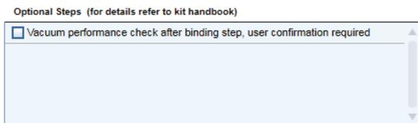
If the vacuum performance check step is activated, the instrument will pause after the binding step. The intermediate step allows to evaluate if all liquid has passed through the membranes. If liquid remains on the surface, re-apply vacuum (**Re-do vacuum**), if not, continue with the procedure (**Proceed**).
