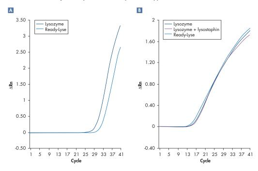
Figure 1 Following pretreatment with the indicated lytic enzymes, bacterial DNA was purified using the MagAttract DNA Mini M48 Kit on the BioRobot M48 workstation. DNA was analyzed on the Applied Biosystems 7500 Real-Time PCR System. A representative amplification plot is shown for DNA purified from group A streptococci (sample 22) and DNA purified from group B streptococci (sample 11).
