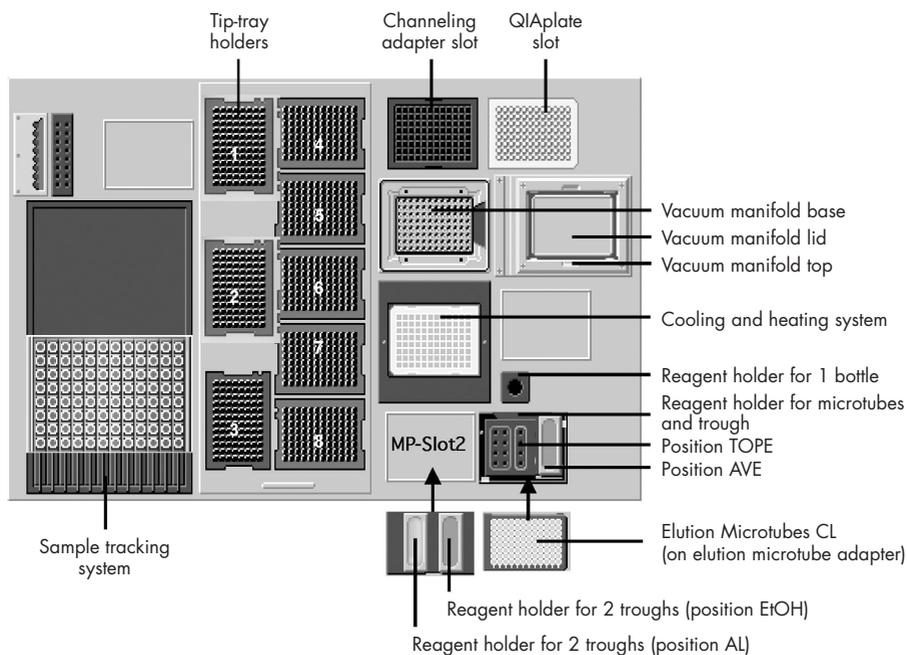
**Figure 1. Overview of the BioRobot MDx worktable and its main components.** Refer to Tables 3, 4, and 5 for more details.
