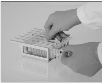
Figure 9. Ease of instrument setup using reagent cartridges (RCB). A sealed, prefilled reagent cartridge (RCB) of the EZ1 DSP DNA Blood Kit. B Loading reagent cartridges (RCB) into the cartridge rack. The cartridge rack itself is labeled with an arrow to indicate the direction in which reagent cartridges (RCB) must be loaded.
