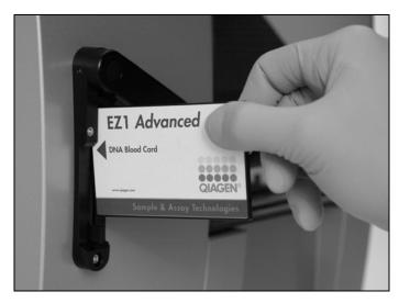
**Figure 7. Ease of protocol setup using EZ1 DSP Cards.** Inserting an EZ1 Card, containing protocol, into the EZ1 instrument.
