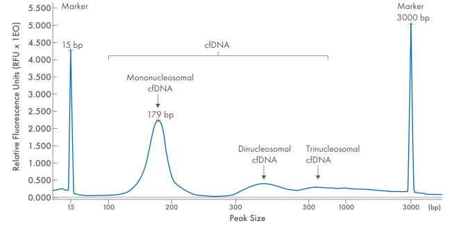
High-sensitivity cfDNA analysis. The sample was extracted from 8 ml plasma using the EZ1&2<sup>™</sup> ccfDNA Kit with EDTA blood collection tubes. The concentration was 0.924 ng/µl (Qubit™ dsDNA HS Assay Kit). QIAxcel Connect facilitates identifying mono-, di-, and trinucleosome peaks, as well as sizing of peaks.
