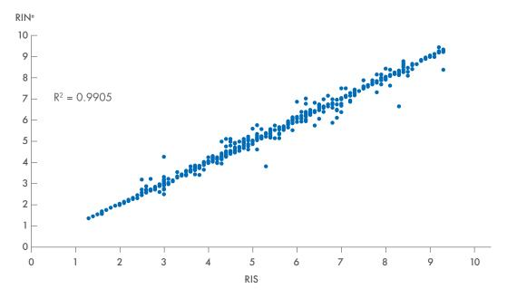
Correlation of RIS and RINe. RNA samples were purified from rat lung, rat liver and Jurkat cells, and then analyzed in replicates (n=689) on the TapeStation 2100 and the QIAxcel system. The RINe and RIS values of the RNA samples were plotted to establish correlation.
