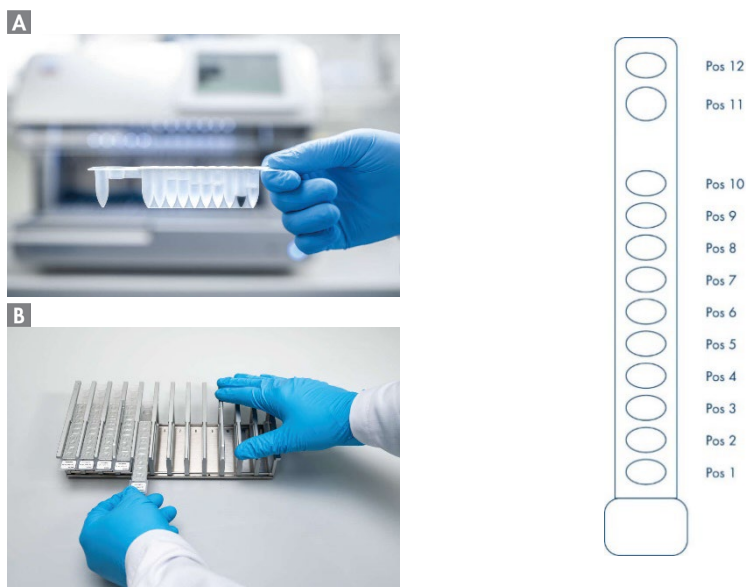
Figure 1. Ease of worktable setup using reagent cartridges. (A) A sealed, prefilled reagent cartridge. Fill levels vary, depending on the type of reagent cartridge. (B) Loading reagent cartridges into the cartridge rack. The cartridge rack itself is labeled with an arrow to indicate the direction in which reagent cartridges must be loaded.
