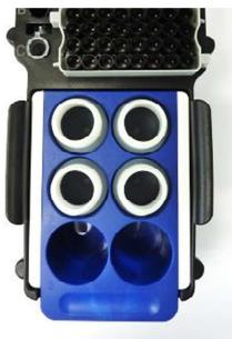
**Figure 2. Reagent Bottle Rack.** Positions 5 and 6 are not used in this protocol.
