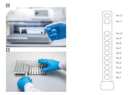
Figure 2. Ease of worktable setup using reagent cartridges. (A) A sealed, prefilled reagent cartridge. Fill levels vary, depending on the type of reagent cartridge. (B) Loading reagent cartridges into the cartridge rack. The cartridge rack itself is labeled with an arrow to indicate the direction in which reagent cartridges must be loaded. Each reagent cartridge contains 12 individual positions.
