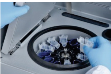
Removing rotor adapters.
