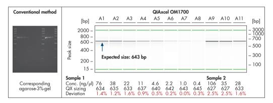
Figure 1. QIAxcel Advanced performs accurate DNA fragment sizing. Gel electrophoresis and fragment sizing of DNA fragments at various concentrations were performed using conventional gel electrophoresis and the QIAxcel Advanced instrument. Locus MIRU10 has repeats of 55 bp. The 643-bp fragment represents 3 alleles.
