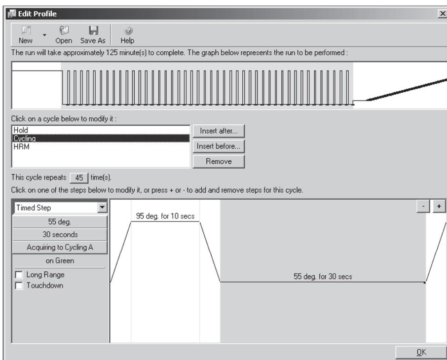
**Figure 8. Two-step cycling.** PCR requires 45 cycles. Each cycle is comprised of 2 steps: 95°C for 10 s (denaturation step) and 55°C for 30 s (annealing/extension step).
