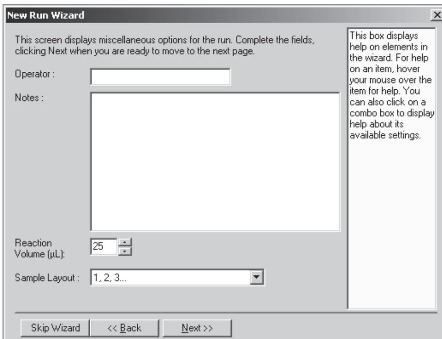
Figure 6. Selecting the reaction volume.
