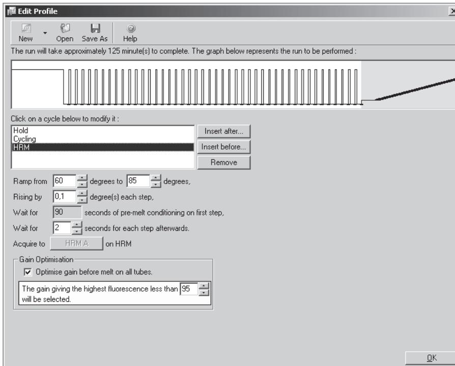
**Figure 9. HRM analysis.** After PCR is completed, HRM analysis can be performed, ramp from 60°C to 85°C, rising by 0.1°C in each step. Ensure that the “Optimize gain before melt on all tubes” check box is checked. Approve by clicking “OK”.
