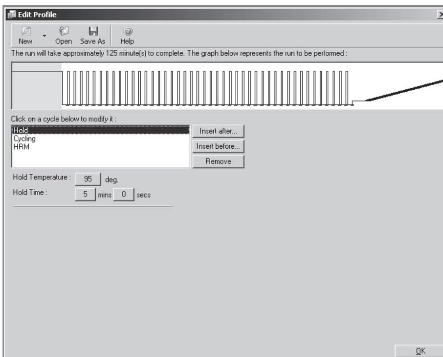
**Figure 7. Initial activation step.** PCR requires an initial incubation at 95°C for 5 min to activate HotStarTaq *Plus* DNA Polymerase.
