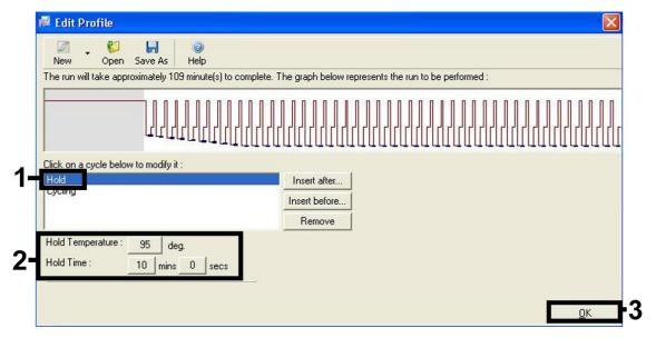
Figure 4. Initial activation of the hot-start enzyme.
