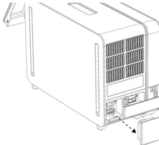
**Figure 12. Removing the Termination Bridge.**
