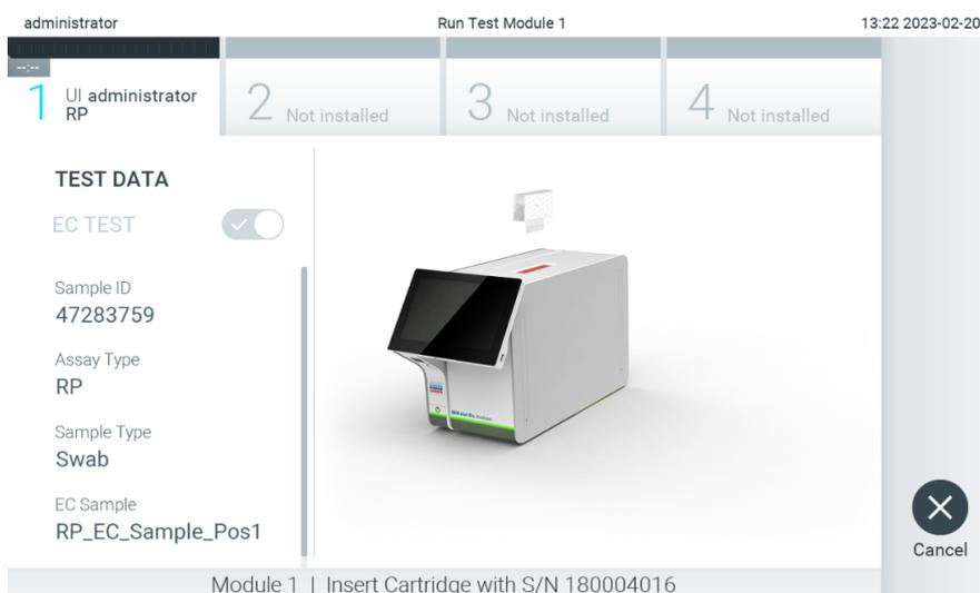
**Figure 97. Inserting QIAstat-Dx assay cartridge into QIAstat-Dx Analyzer 2.0.**
