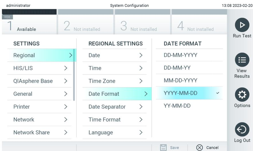
**Figure 61. Setting the system date format.**
