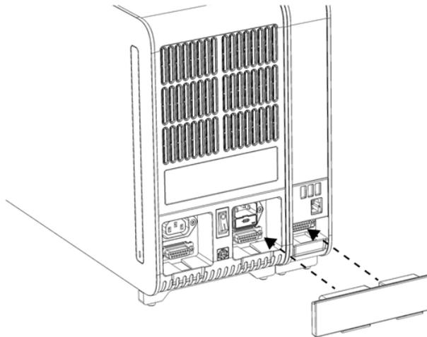
**Figure 8. Connecting the Analytical/Operational Module Bridge.**
