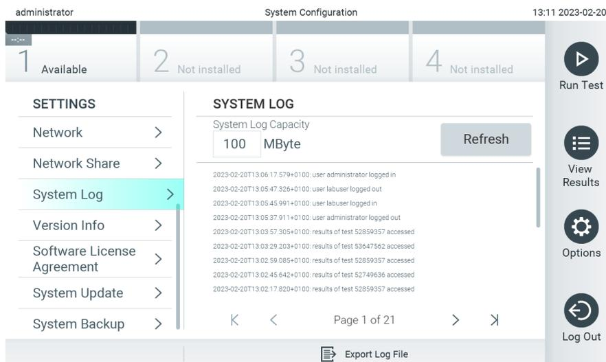
**Figure 69. Accessing the system log.**
