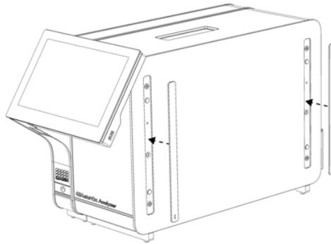
**Figure 7. Reattaching the protective covers.**
