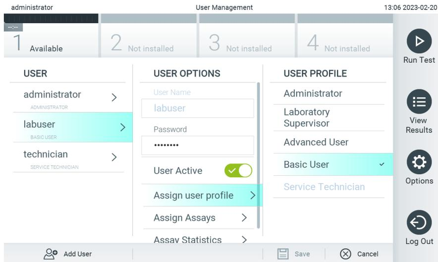
Figure 52. Assigning user profiles to users.
