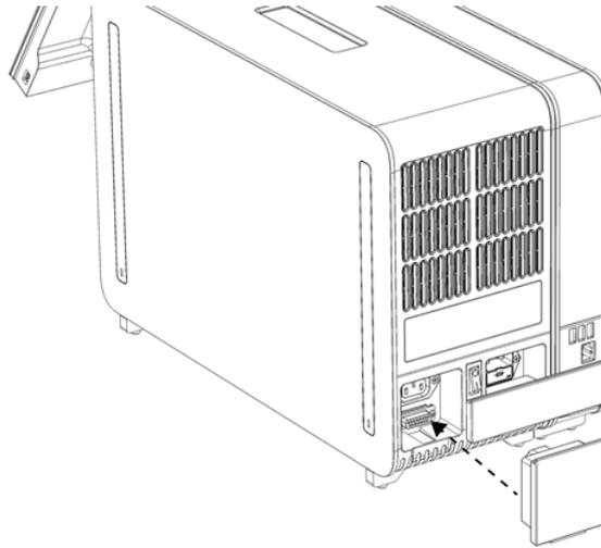
**Figure 9. Connecting the Termination Bridge.**
