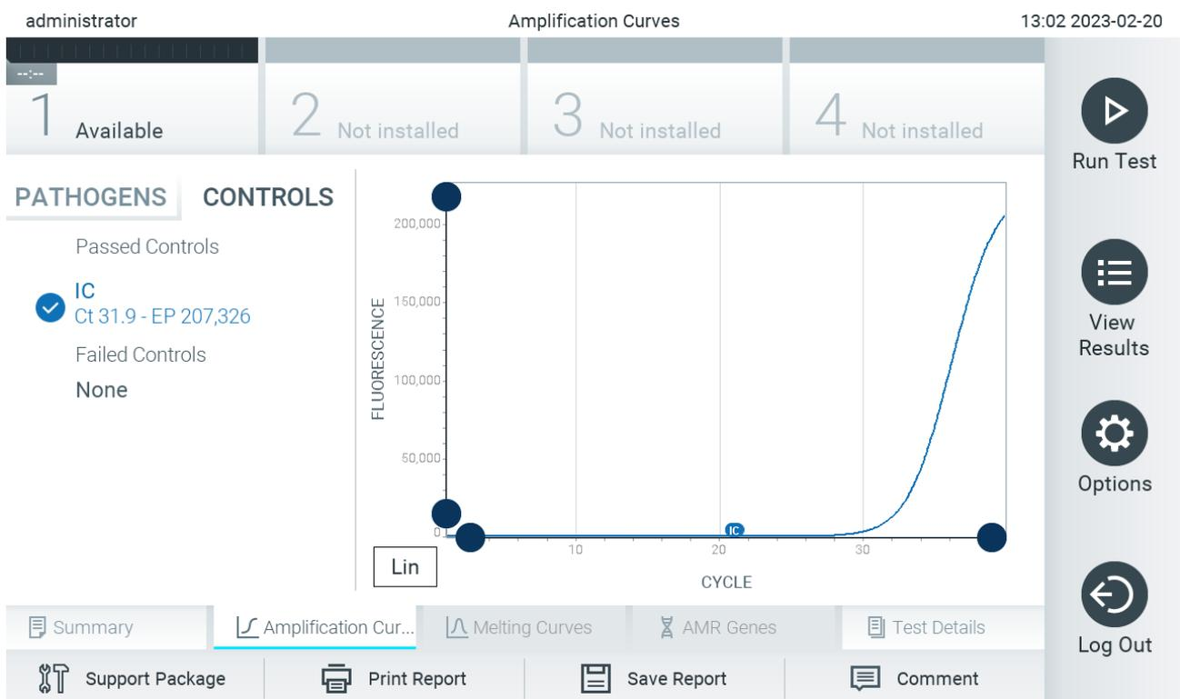
Figure 35. Amplification Curves screen (CONTROLS tab) showing internal control.
