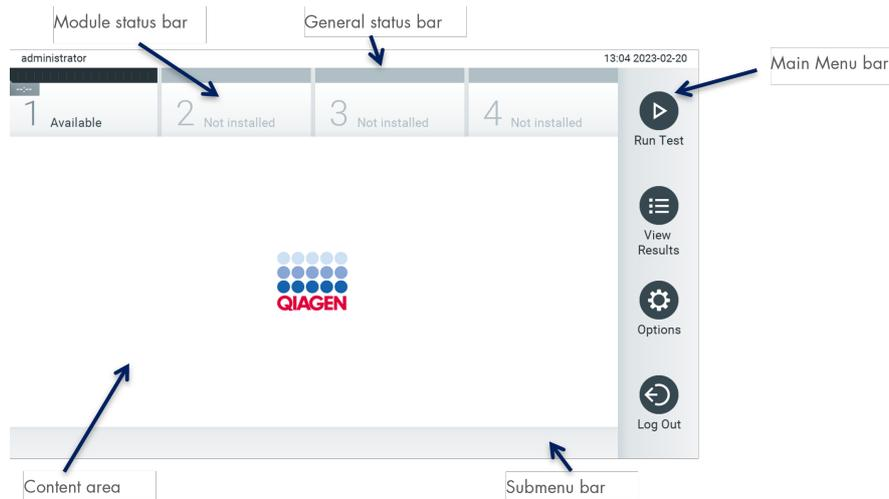
Figure 42. Main screen of the QIAstat-Dx Analyzer 2.0 touchscreen.
