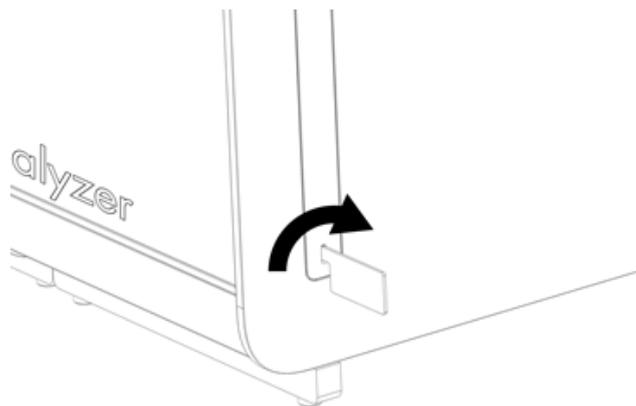
**Figure 13. Removing protective covers.**
