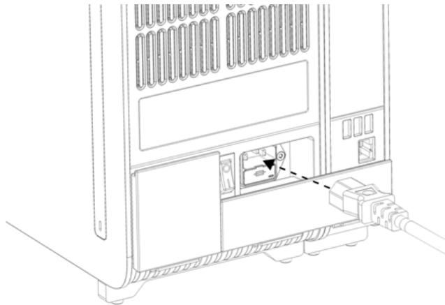
**Figure 20. Connecting the power cord.**
