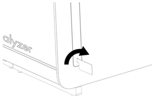
**Figure 15. Removing protective covers.**
