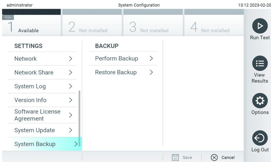
**Figure 71. Performing a system backup.**
