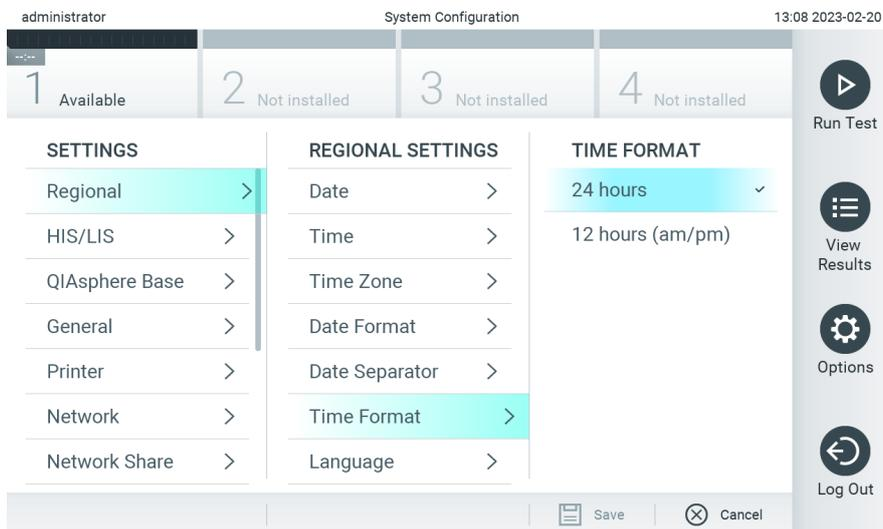
Figure 63. Setting the system time format.
