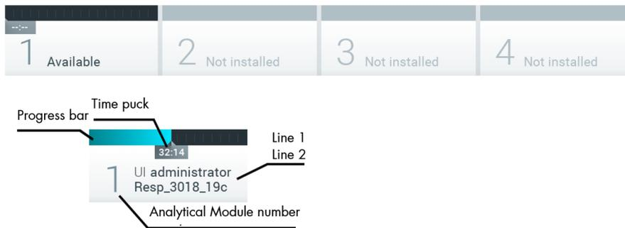
Figure 44. Module status bar.
