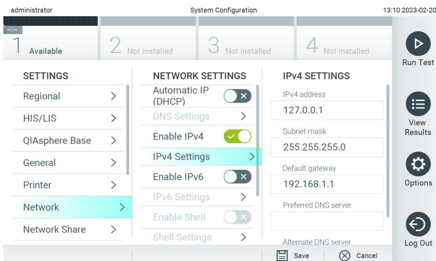
Figure 67. Configuring the network settings.
