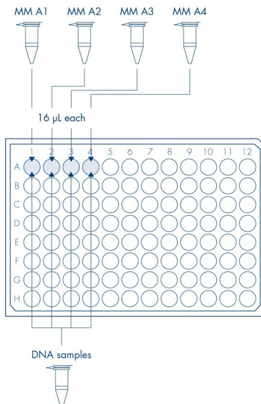
**Figure 6. Example of a 4-pool panel.** DNA samples have already been aliquoted into wells in step 3. **Do not add anymore DNA.**
