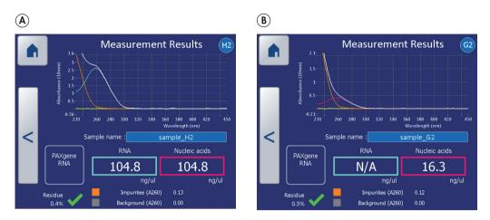
Figure 2. Example result screen for spectral content analysis. RNA was purified from human whole blood using the QIAsymphony PAXgene Blood RNA MDx Kit and the QIAxpert PAXgene RNA App was used for measurement. **A** An RNA-profiled PAXgene RNA sample with an RNA concentration of 104.8  $g/\mu$ l and a low residue value of 0.4%. **B** A PAXgene RNA sample, where RNA profiling is unavailable, due to a low nucleic acid concentration of 16.3  $g/\mu$ l, but still showing a low residue value of 0.5%.
