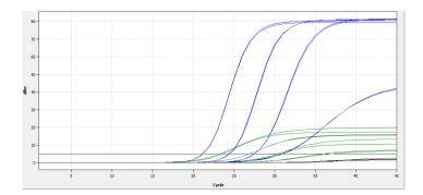
Figure 2. Amplification plots showing strong signals in the FAM channel (blue curves) that bleed into the adjacent channel (JOE-green curves). Color compensation off.
