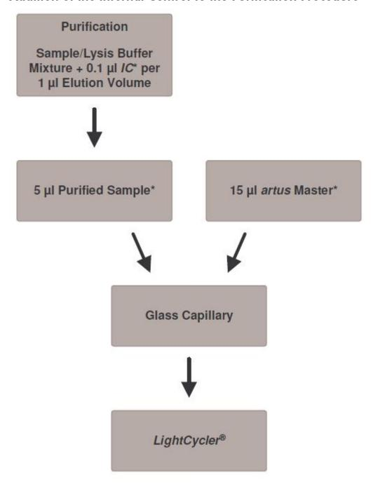
Fig. 1: Schematic workflow for the control of both the purification procedure and PCR inhibition.
