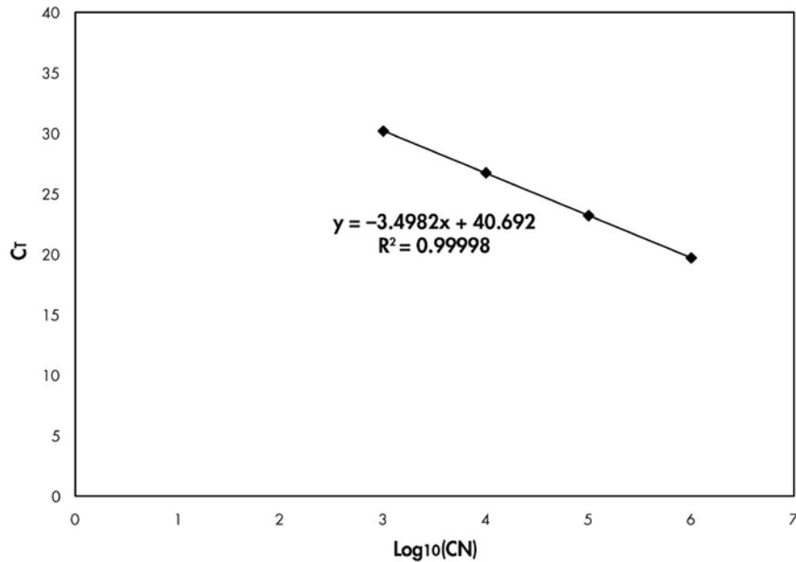
**Figure 9. Theoretical standard curve for ABL calculated from 4 standard dilutions.** A linear regression curve ( $y = ax + b$ ) is calculated, where  $a$  is the slope of the line and  $b$  is the  $y$ -intercept, which is the  $y$ -coordinate of the point where the line crosses the  $y$  axis. Its equation and coefficient of determination ( $R^2$ ) are printed on the graph.
