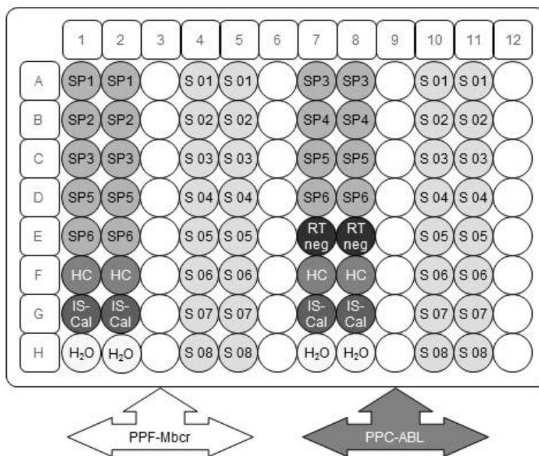
**Figure 5. Suggested plate setup for one experiment with the *ipsogen* BCR-ABL1 MbcR IS-MMR Kit. SP1–SP6:** BCR-ABL MbcR and ABL standards; **HC:** High cDNA positive control; **IS-Cal:** IS-MMR calibrator; **RTneg:** RT negative control; **S:** cDNA sample; **H<sub>2</sub>O:** water control.
