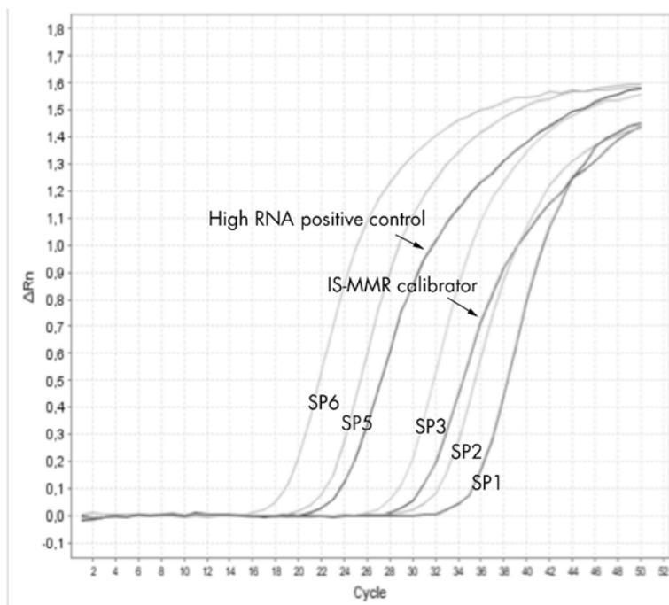
**Figure 8. Detection of BCR-ABL MbcR with standards SP1, SP2, SP3, SP5, and SP6.**  $10^1$ ,  $10^2$ ,  $10^3$ ,  $10^5$ ,  $10^6$  copies/ $5 \mu\text{l}$ .
