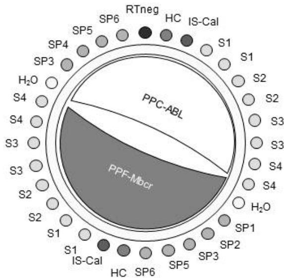
**Figure 6. Suggested rotor setup for each experiment with the ipsogen BCR-ABL1 Mbcr IS-MMR Kit. SP1–SP6:** BCR-ABL Mbcr and ABL standards; **HC:** High cDNA positive control; **IS-Cal:** IS-MMR calibrator; **RTneg:** RT negative control; **S:** cDNA sample; **H<sub>2</sub>O:** water control.
