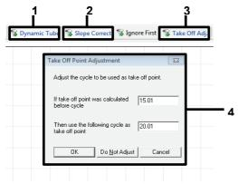
**Figure 13. EGFR analysis normalization settings.** 1 = "Dynamic Tube," 2 = "Slope Correct," 3 = "Take Off Adj," 4 = "Take Off Adj" dialog window with parameter values.
