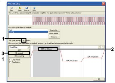
Figure 6. Cycling step at 95°C.
