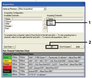
Figure 8. Acquiring at cycling step of 60°C.
