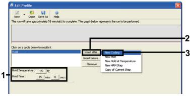
Figure 5. Initial incubation step at 95°C.
