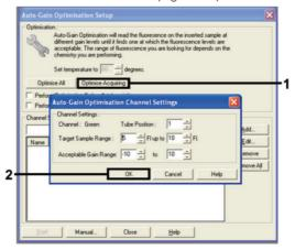
Figure 11. Auto-gain optimization for the Green channel.
