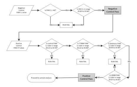
Figure 14. Run control analysis workflow.
