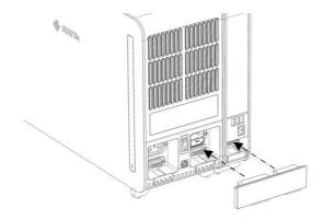
6. Connect the termination bridge at the back of the Analytical Module.
