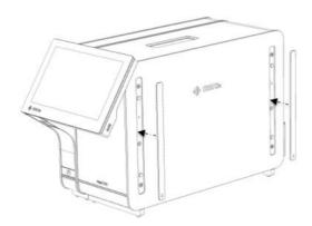
5. Connect the Analytical/Operational Module bridge at the back of the DiagCORE Analyzer to link the Operational and Analytical Modules together.
