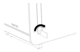
3. Remove the Operational Module from its box and attach it to the left side of the Analytical Module. Tighten the screws using the Analytical-Operational Module assembly tool delivered with the DiagCORE Analyzer.
