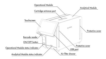
Front view of the DiagCORE Analyzer. The Operational Module is on the left, and the Analytical Module is on the right.
