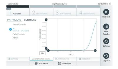
Amplification Curves screen showing the Controls tab.
