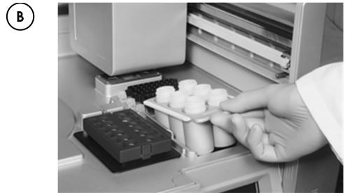
**Figure 4. Loading the reagent bottle rack.** [A] Schematic of positions and contents of bottles in the reagent bottle rack. [B] Loading the rack onto the QIAcube Connect.
