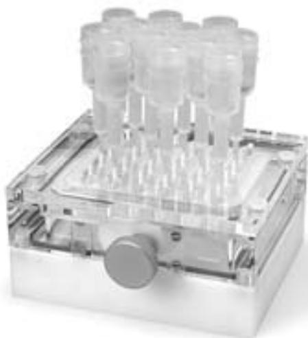
**Figure 5.** Ni-NTA Superflow Columns on the BioRobot vacuum manifold. Columns are processed in multiples of 4; up to 12 columns can be processed per manifold.
