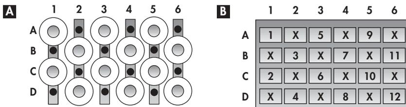
**Figure 6.** **A** Positioning of Ni-NTA Superflow Columns on Luer Adapter Strips on the QIAvac 6S Top Plate. **B** Elution fractions (1–12) are collected in the indicated wells of a 24-well block.
