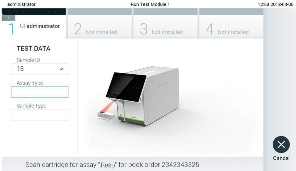
Figure 83. Scanning the QIAstat-Dx assay cartridge bar code.
