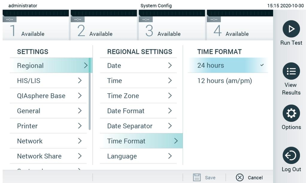
Figure 71. Setting the system time format.
