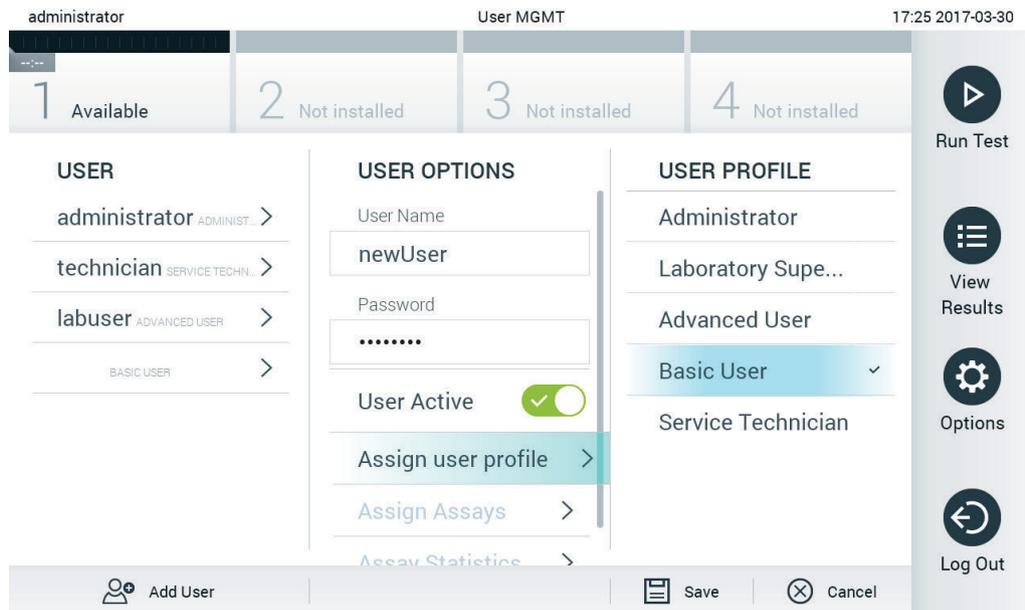
Figure 64. Assigning a user profile to a new user.
