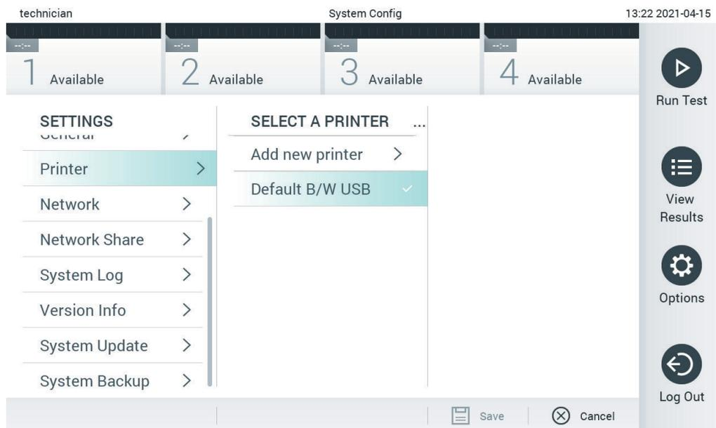
Figure 73. Selecting a system printer.
