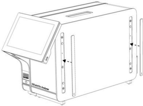
Figure 7. Reattaching the protective covers.
