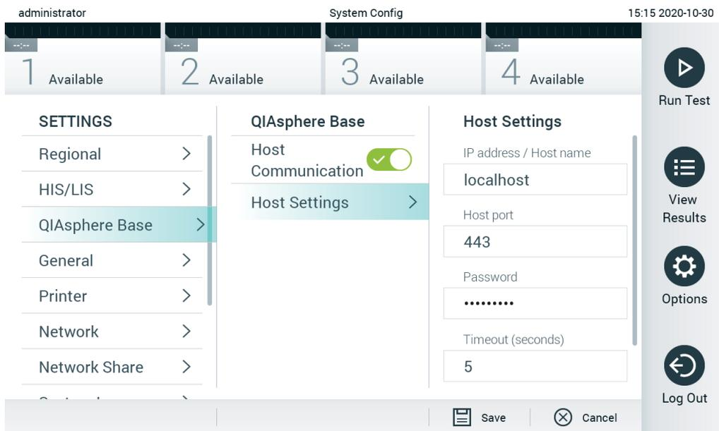
Figure 72. Configuring the QIAsphere Base connection.
