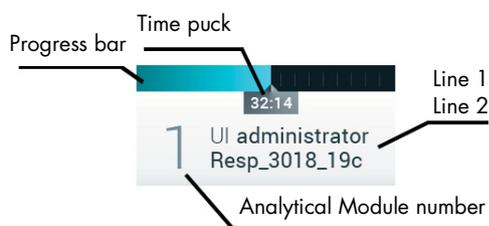
Figure 43. Module status bar.
