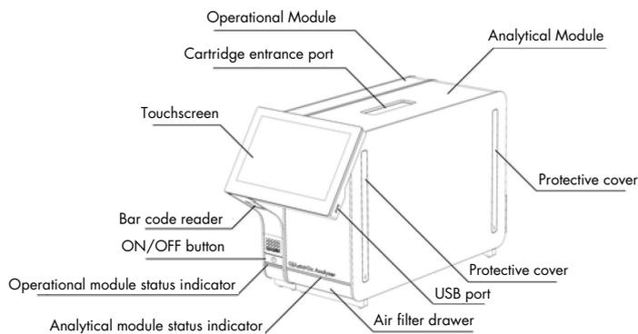
**Figure 1. Front view of the QIAstat-Dx Analyzer 1.0.** The Operational Module is on the left and the Analytical Module is on the right.
