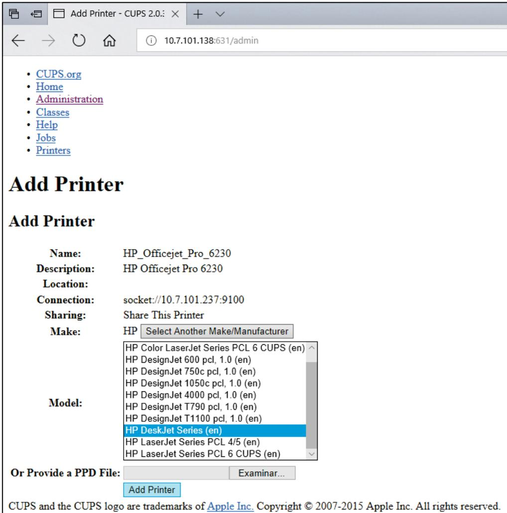
Figure 102. Selecting the printer driver.
