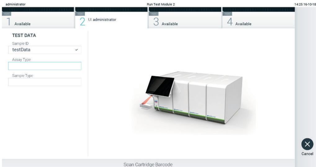
Figure 24. Scanning the QIAstat-Dx assay cartridge bar code.
