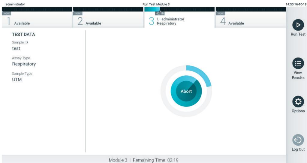
Figure 28. Test execution and remaining run time display.
