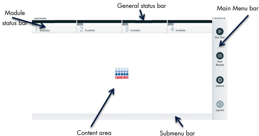
Figure 41. Main screen of the QIAstat-Dx Analyzer 1.0 touchscreen.
