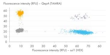
Figure 5. Strong signal separation between channels in multiplex. 2D scatter plots of various dye combinations from 4-plex multiplex runs. Four assays targeting four bacterial resistance genes were run in multiplex reactions using 26k 24-well Nanoplates and the QIAcuity Probe PCR Kit on the QIAcuity Digital PCR System.
