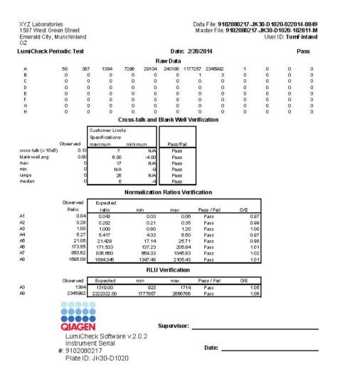
The header of the LumiCheck periodic test report includes the laboratory header information. See "Modifying the laboratory header information," page 47, for instructions to change the laboratory header information.
